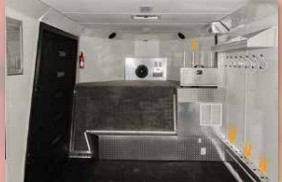
Ducted Heat Option to Dry Boots, Gloves, Coats, Bibs and Helmets
