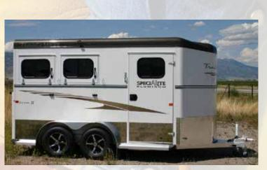
Factory applied Polyurethane paint and Epoxy primer, Two-tone roof/body paint with roof rail color choices of Silver, Charcoal, Black, or Cypress Gold (SpeciALite models only), Drop down feed doors, Sliding tail side windows, Double rear doors with windows, Roof vent in each stall, Horse compartment roof lined and insulated, Swing-out saddle rack, Swing-out blanket rack, LED marker and tail lights, Aluminum wheels, Choice of graphics.
